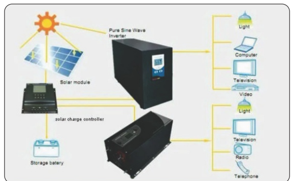
SOLAR UPS SYSTEM
